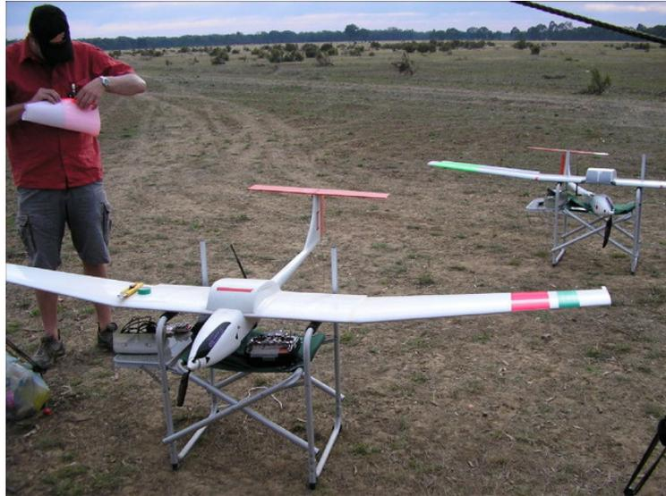
**Figure 1. Team vehicles undergoing communications tests prior to launch**
