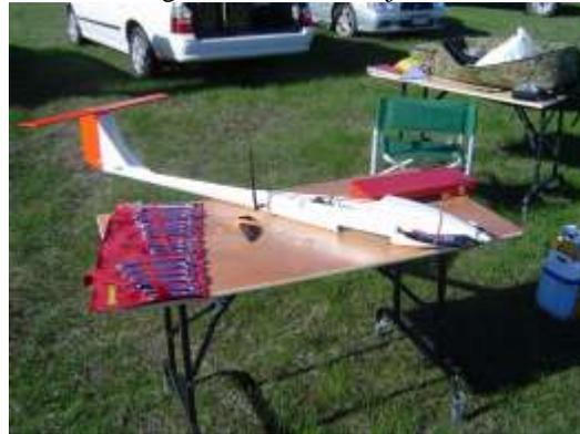
**Figure 2: The Codarra Avatar prior to assembly for launch. The cavity for the payload bay is visible on the underside of the aircraft and the wireless modem aerial can be seen standing vertically. The prop is fully folded, as it can be in flight, along the fuselage.**
