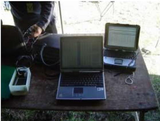
**Figure 1: From left to right: the payload bay containing the IPAQ; the notebook for loading the Intelligent Agent waypoints into the IPAQ; and the Avatar Ground Control Station (GCS).**
